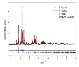
**Figure 5.** Rietveld refinement profile of the x-ray powder diffraction data for sample 3. Tick marks indicate reflections coming from the majority phase  $La_5Si_3$ .
