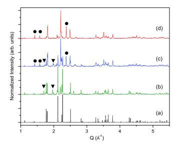
**Figure 3.** X-ray diffraction patterns of the four different samples: 1 (a), 2 (b), 3 (c) and 4 (d). The  $\bullet$  indicate diffraction maxima from La<sub>5</sub>Si<sub>3</sub> and the  $\blacktriangledown$  indicate those coming from La<sub>2</sub>C<sub>3</sub>.
